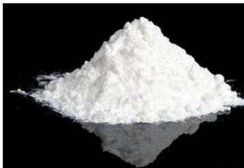
Titanium (IV) oxide for fiber optics chemical purity 99.999% is a white or slightly yellow finely dispersed powder, insoluble in water, dilute sulfuric, nitric and hydrochloric acids. Goods is soluble in hydrofluoric acid and in molten borax.
